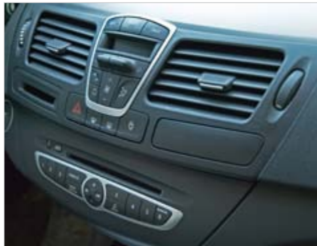
Polycarbonate made from isosorbide for the automobile market
